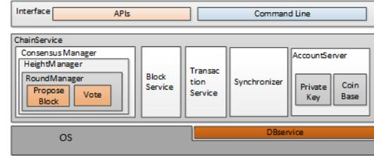
Figure 2: HydraChain Architecture
